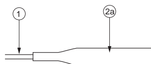
Style 34 1: 75 cm capillary 2: 1/4" tube for braze connection
