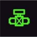
**OUTPUT STATUS ICON** EEV Output status for the electronic valve EEV (if enabled)
