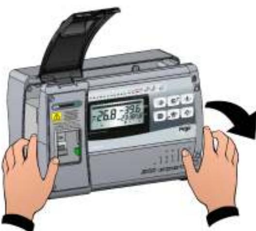
**Fig. 3:** Open the front of the box, lift it and slide the two hinges out as far as they will go. Bend the hinges and rotate the front panel by 180° downward to get access inside the panel
