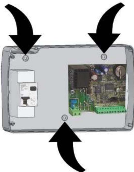
**Fig. 6:** Use the three existing holes to fix the box back panel to the wall: use three screws of a length suitable for the thickness of the wall to which the panel will be attached. Fit a rubber washer (supplied) between each screw and the box backing.
